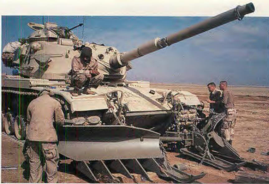
A Pearson Engineering track-width mine plow is hastily attached to M-60 tank prior to ground offensive. Photo: Sygma/Langevin
