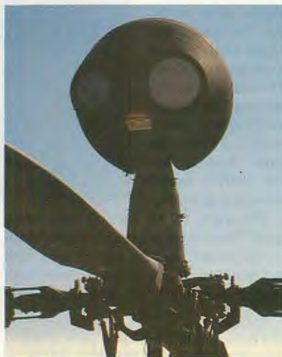
Mast-mounted laser range finder designator.
