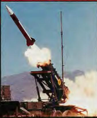
Built by Raytheon and Martin Marietta, the Patriot's fast reaction capability and ability to operate in a severe electronic countermeasure environment are features that set it apart from systems it is replacing. Photo: U.S. Army/Frank Trevino
