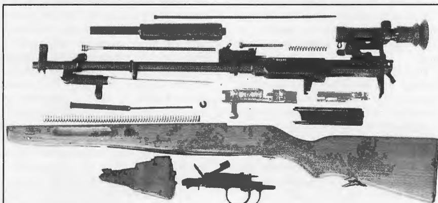
"Para" SKS with Type 89 scope — field stripped.
