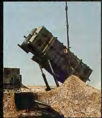
Each Patriot station has four missiles and a trailer (under camouflage netting) housing radar equipment. Photo: DoD
