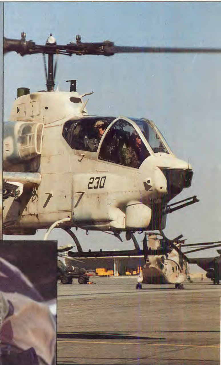
ABOVE: Business end of Marine SuperCobra sports three-barreled 20mm cannon, but craft is primarily a mobile missile launcher, carrying Hellfire, TOW and AIM-9 Sidewinder missiles for whatever it meets on land or in air. Photo: Ross Simpson
