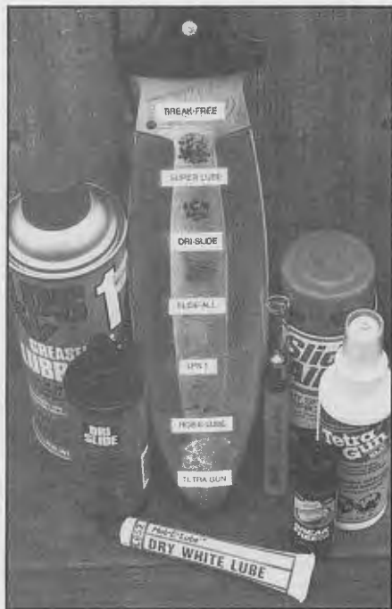
SOF tested all lubes for dust retention by applying them to metal surfaces and dusting with sand/dirt mix. Least amount of dirt was retained by Slide-All, most by Break Free. Photo: SOF staff
