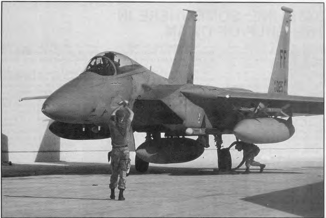
F-15 Eagle fighter ready for action. Sun heats skin of F-15 expanding metal and creating fuel leaks. Dust and fog often shroud potential battlefields, reducing visibility to below 10 klicks. Windy cold fronts, starting in November, pick up huge quantities of dust and can reduce visibility to below 1,000 meters. Photo: DoD
