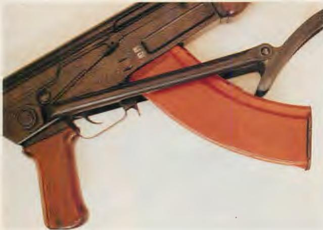
Closeup of North Korean AK-47 downfolder with Soviet-made red plastic magazine.
