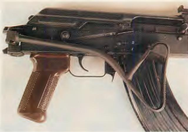
Closeup of East German MPiKMS-72 manufactured in 1984 shows selector markings of 'D' ("dauerfeuer" for full auto) and 'E' ("einzelfeuer" for semiauto) and details of its unique folding stock.
