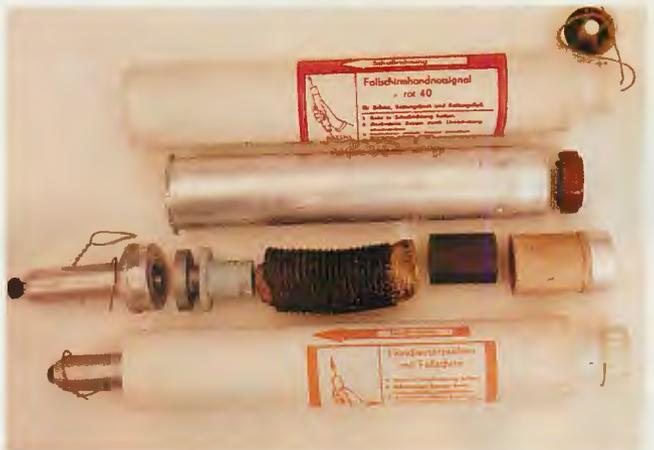
Improvised "flare bombs" are fabricated from German parachute flares modified by the addition of a wire-wrapped charge of the plastic explosive Flex-X.
