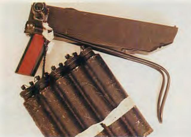
Designed for use against helicopters, parachute flares filled with wire-wrapped Flex-X can be fired singly by pull-cord or by means of this shoulder-held nine-tube launcher. The maximum effective range is 600 to 700 meters.
