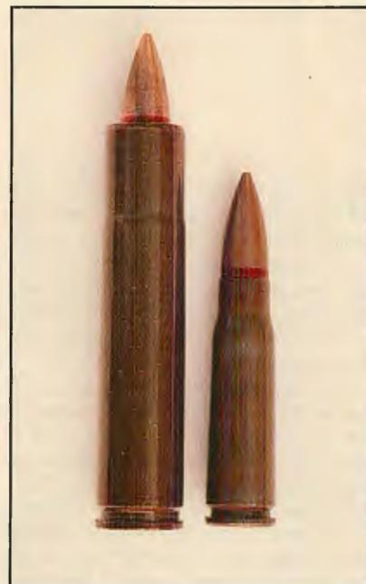
ABOVE: 7.62x62.8mm low-signature cartridge (left) shown in comparison with standard Soviet-manufactured 7.62x39 ball round used in Kalashnikov. Note similarity of case mouth sealants and case lacquers. Photo: Peter G. Kokalis
