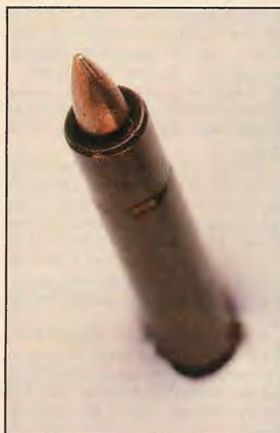
7.62x62.8mm cartridge case is beveled at the mouth and 2.46mm thick in this area to withstand the radial stresses which occur at the internal stop shoulder when it is impacted by the piston within the case. Photo: Peter G. Kokalis
