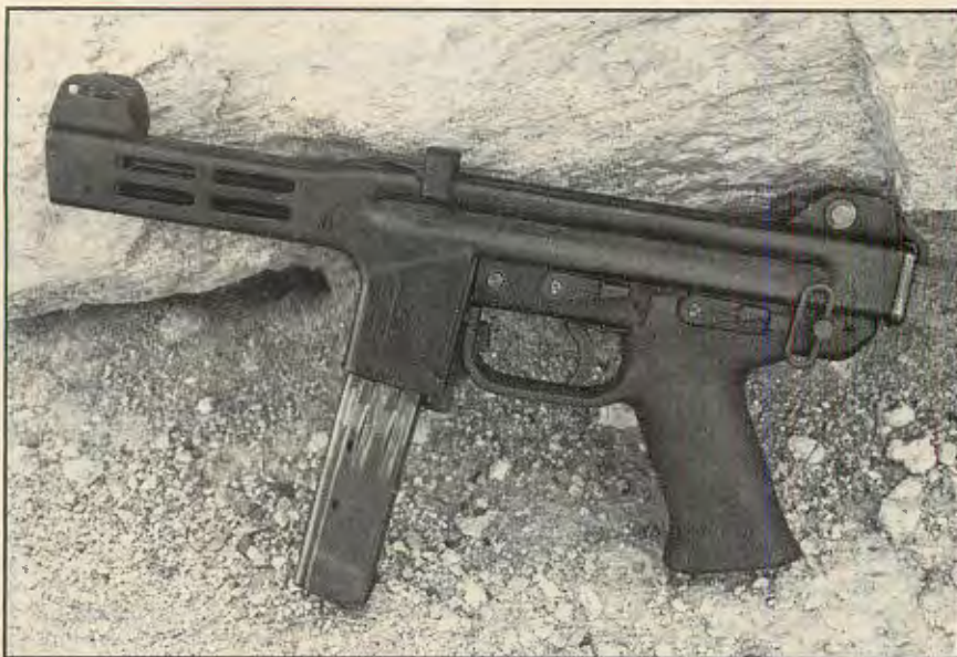
Spectre HC pistol with 30-round magazine. Note safety lever above trigger and de-cocking lever to the rear. Both are ambidextrous. Trigger pull weights vary from 2 pounds in single-action to 14.5 pounds in double-action.
