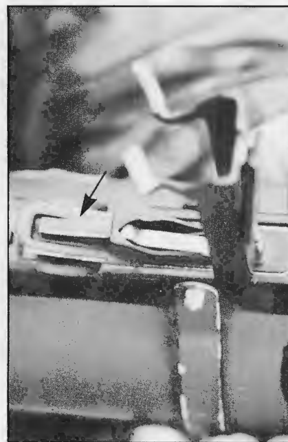
BELOW: Temperature-adjustment assembly and firing guard are lifted to expose the firing lever (arrow).
