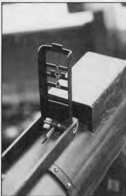
BELOW: Front sight is graduated from 50 to 250 meters.
