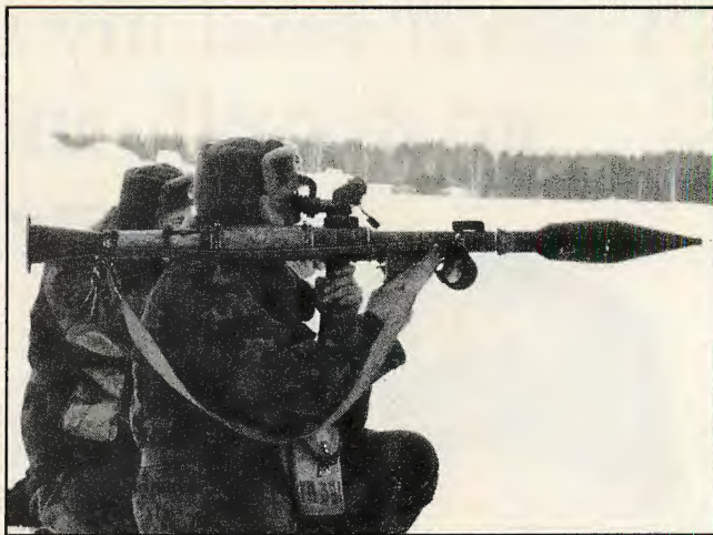
ABOVE: RPG-7D (break-down version of the RPD-7) is still the favorite anti-armor weapon of the VDV (airborne) and VSN (Spetsnaz) troops as it is reusable, and each trooper can carry one or two rounds — still lighter than the same number of disposable RPGs.
