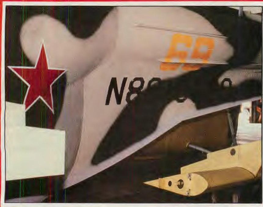
ABOVE: Front view of one of the first operational Hind look-alikes. Note details like missile detector pod (lower right) and air data boom (protruding out front).
