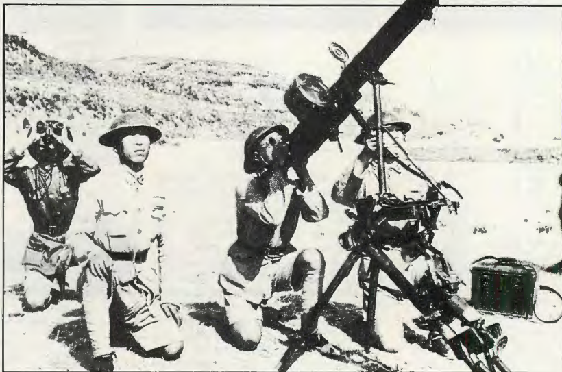
Chinese gun crew with their Type 24 Maxim set up for AA firing. Note the drum magazine, AA extension and ring-type AA sight. Photo: courtesy Robert W. Faris
