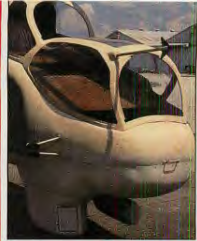
ABOVE: Front view of one of the first operational Hind look-alikes. Note details like missile detector pod (lower right) and air data boom (protruding out front).
