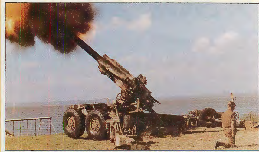
ABOVE: South African G5 155mm towed gun as used in the indirect-fire role.
