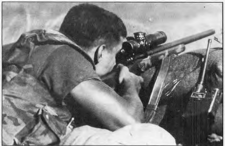
L/Cpl Tom Rutter sights through Unertl scope at sniper position. Note large windage and elevation knobs, camouflaged fiberglass stock on M40 sniper rifle, hand-built by Marine Corps on Remington 700 action. Photo: courtesy Tom Rutter
