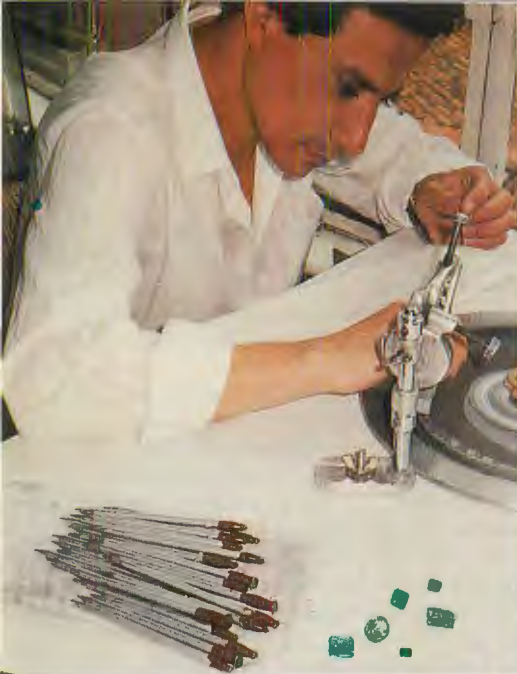
ABOVE: The raw stones are chemically cleaned, then faceted on a diamond lap. Small stone at lower right is worth more than larger stones in picture (approx. U.S. $9,000 according to company), because of its clarity and deep color.
