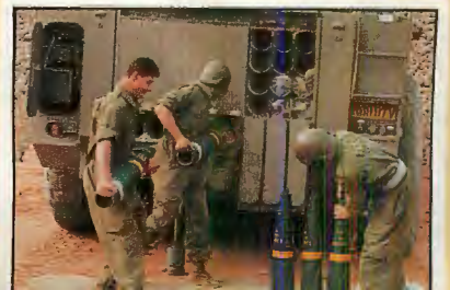
BELOW: Emergency ammunition supply for the G6 Rhino is stored in a compartment at the rear of the hull which is provided with blow-off doors.
