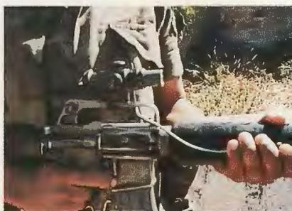
**ABOVE:** Airborne sniper holds M16A1-mounted IR laser target designator author discusses in article. Wearing IR goggles, sniper need only track laser beam to target. Conventional sighting is not required. Although it *looks* like a scope, it is an IR laser projector. These devices were without any markings — they could be either sterile or prototypes — but author's guess as to manufacturer is Litton.
