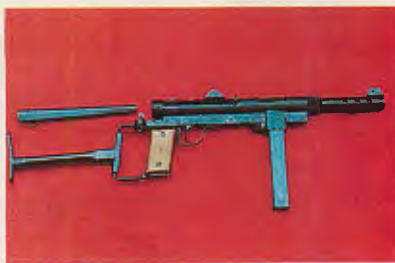
This unusual variant of the Swedish 'K' — the M45BE — was issued to Swedish police. The stock was redesigned because police ballistic helmets inhibited sight acquisition. Note clip-on cheekpiece for use when helmets were not worn. This model also had a selector lever that permitted semiauto fire. Photo: Jan B. Borjesson
