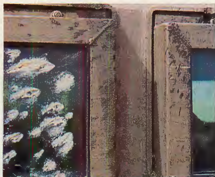
PG-7 antitank grenades will penetrate the Casspir MPV's unitary armored hull. Note fragment splatter on left window; shaped charge's collapsed copper cone punched hole above right window.
