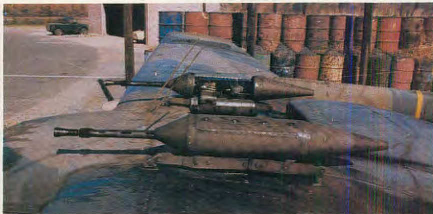
TOP: Sanctions-busting Lynx, Fire Force's air-ground attack aircraft, carried two top-mounted .303 machine guns, and a variety of ordnance including frantan (napalm), rockets, and Rhodesian-manufactured fragmentation bombs. Photo: courtesy author
