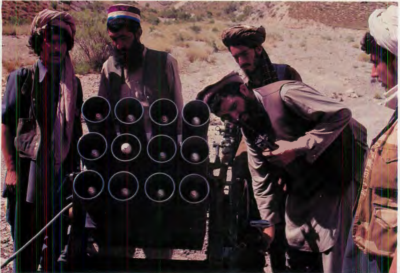
Business end of a 12-tube 107mm Type 63 multiple rocket launcher, with rockets visible in tubes. Type 63s have since been augmented by more powerful 122mm Sakr system. Photo: Sayd Ehsanullah
