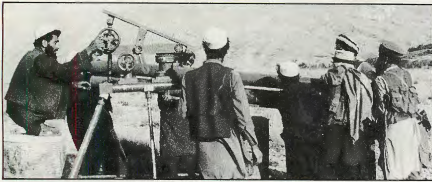
The four firing tubes of a Sakr launcher being positioned on tripod, the light legs of which are visible in photo. The whole assembly can be moved by mule or jeep. Photo: Afghan Media Resource Center
