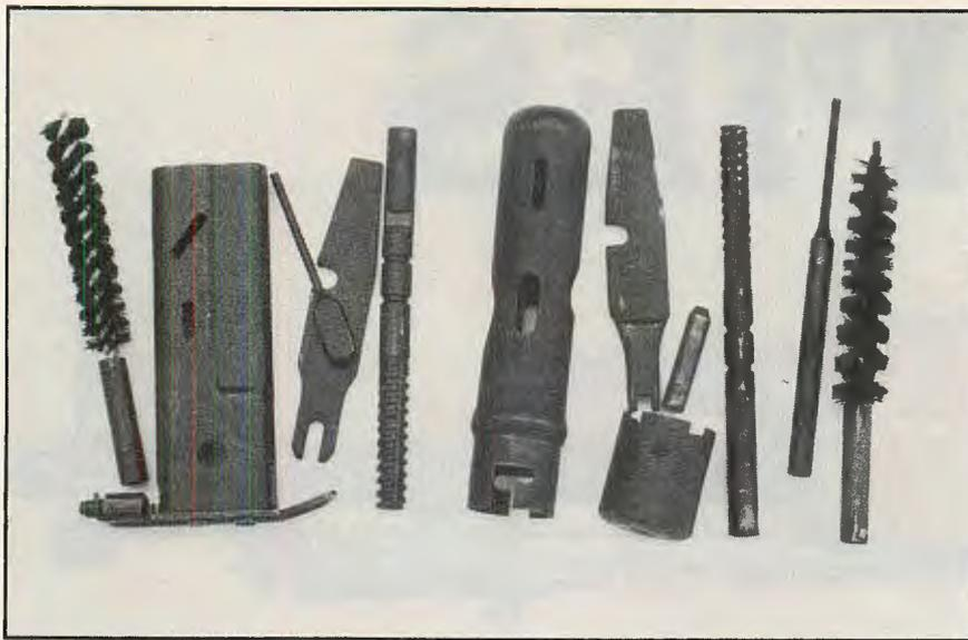
**Kalashnikov cleaning kits. On the left for the PRC Type 56-2 sidefolder and on the right is a typical AK-47/AKM buttstock cleaning kit.**
