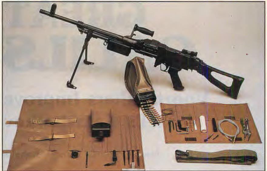
SS-77 GPMG in its final production series configuration, complete with cleaning and maintenance kits, sling and assault pack. Photo: courtesy Lyttelton Engineering Works
