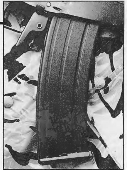
New synthetic 35-round magazine for the R4 will replace older and much heavier steel magazines. More durable and just as reliable, it can be produced for half the cost.
