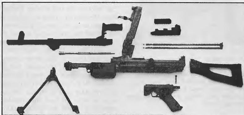
Production model SS-77 GPMG field stripped.
