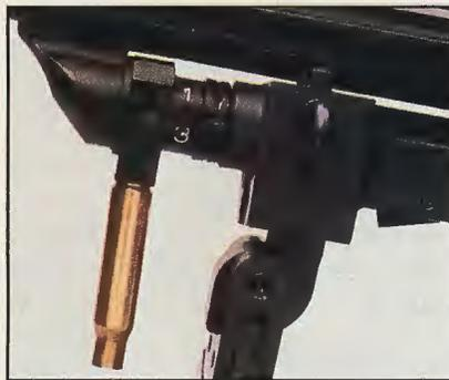
SS-77's gas system has been taken directly from that of the Soviet PKM, except that the gas vent has been drilled at a 57-degree angle to the bore's axis to permit cleaning. Gas regulator is adjusted by means of an empty cartridge case. Photo: courtesy Lyttelton Engineering Works
