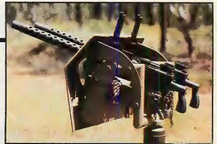
Flexible twin mounting of MG4 AA. Now firing from open bolt position, this 7.62x51mm NATO caliber conversion is most commonly employed on armored fighting vehicles. In this role it's as good as it ever was — and still better than most.
