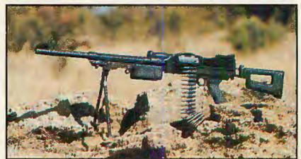
SS-77 GPMG shown with intermediate prototype buttstock and longitudinal cooling fins on barrel. Photo: courtesy Armscor
