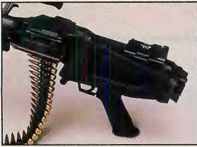
SS-77's left-folding buttstock is injection-molded over two steel pins which are integral with the investment-cast hinge mechanism. Note the thick recoil pad which reduces perceived recoil to an almost unnoticeable level. Photo: courtesy Lyttelton Engineering Works
