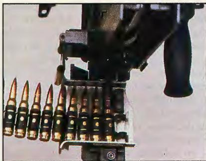
SS-77 stainless steel feed tray. Note slots on the tray which help to retain the RIM1 links. Photo: courtesy Lyttelton Engineering Works
