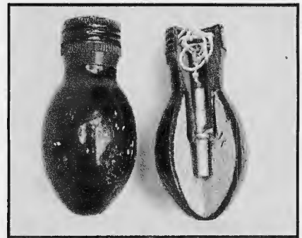
ABOVE: The oval-shaped PRC Type 82-1 grenade has an atavistic pull-friction fuze and an inner liner with hexagonal serrations.
