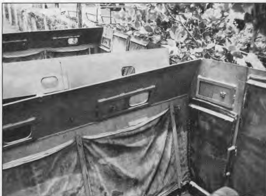
ABOVE: Close-up of soldier's post on the troop-carrier version of Cashuat. Note sliding gun ports and the ballistic nylon tacked up to stop projectiles if they manage to penetrate the outer armor. Photo: David E. Spencer
