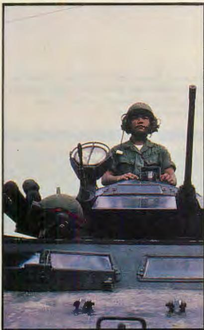
This Cadillac Gage Commando V-150 armored vehicle is armed with a .50-caliber HMG and an M60 machine gun. Various versions of the V-150 provide most of the armored firepower for the Philippine armed forces.
