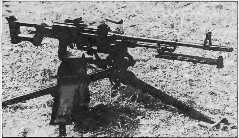
PRC Type 80 GPMG mounted to its 10.4-pound aluminum tripod.
