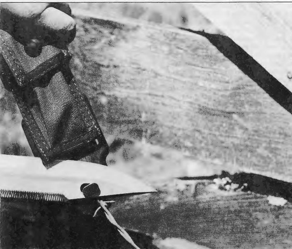
One of Army's major specifications required the M9 to cut wire like its Soviet counterpart. However, it's awkward, inefficient and tactically unsound as a wire cutter, requiring two hands to operate. And incidentally, watch your fingers!
