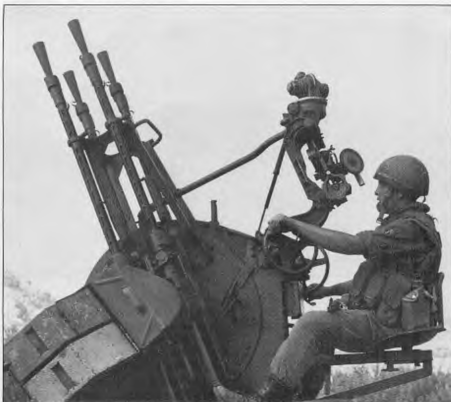
ABOVE: Antiaircraft weapons like this ZPU-4 14.5mm heavy machine gun spend time busting buildings, bunkers, trucks, APCs and an occasional aerial target.
