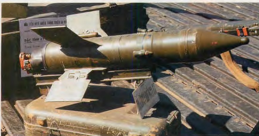
ABOVE: Soviet Sagger antitank missiles captured from the NVA. Photo: Ed Besch
