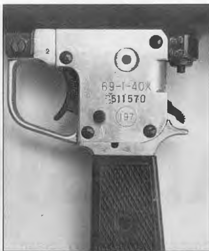
Type 69 pistol grip and trigger group. Hammer is in cocked position, ready to strike firing pin mechanism directly above it.
