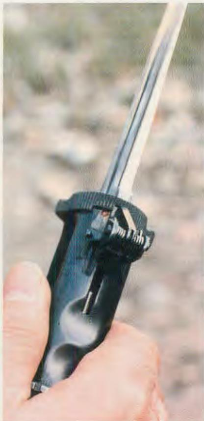
**ABOVE:** Red dot on safety ring of trigger/crossguard means knife pistol is ready to "fire." Note front sight just to left of trigger pivot and return spring.
