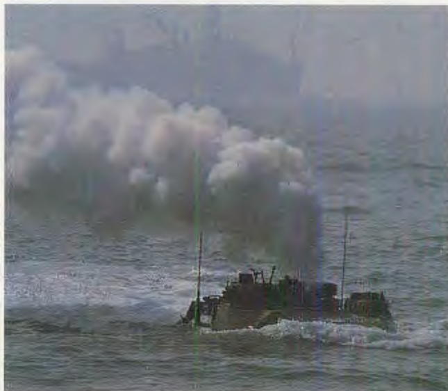
BELOW: An AAV7A1, or amtrac, capable of carrying 25 combat-loaded Marines, nears the beach.
