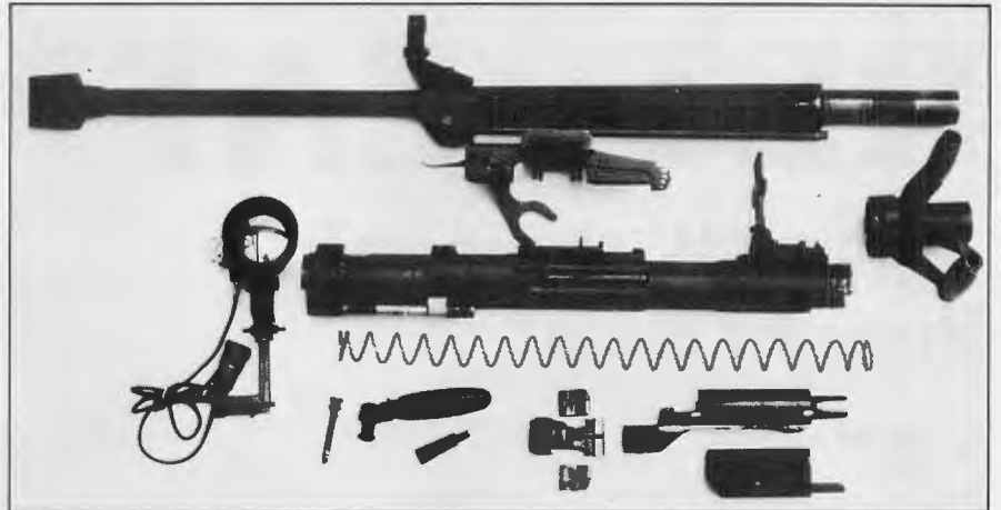
ABOVE: Type 77 muzzle brake effectively controls muzzle climb and flash, but its blast sends up swirling clouds of dust when the weapon is fired from the low prone position.
