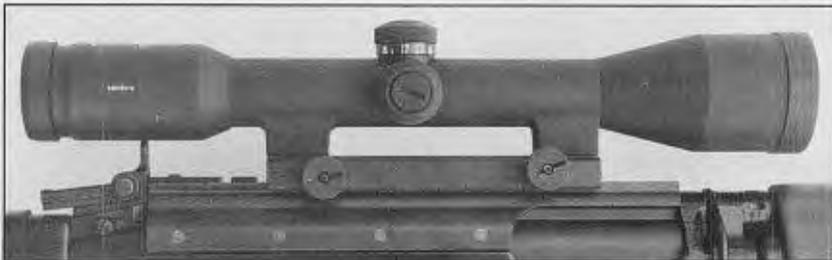
**Swarovski RZFM-6 6x42mm scope features reticle rangefinder patterned after Dragunov/RPG-7. Mounted to FN FAL by means of A.R.M.S. mount which completely replaces FAL's sheet-metal receiver cover.**
