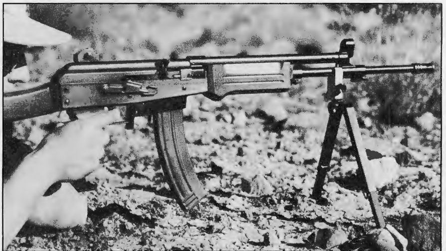
Galil-22 with optional bipod that can be attached to any number of rifles.
