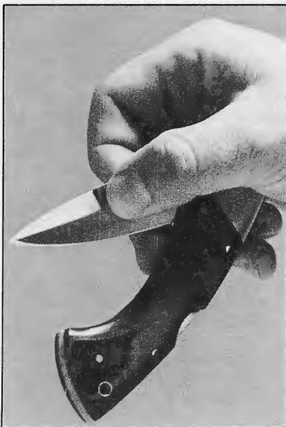
The largest disadvantage is the folding lockback's inherent mechanical weakness. A lockback is dependent on three key components to hold it open: the pivot pin, lock mechanism and back spring. Any one, or all three, of these parts can be overcome or broken under the strain of combat.
