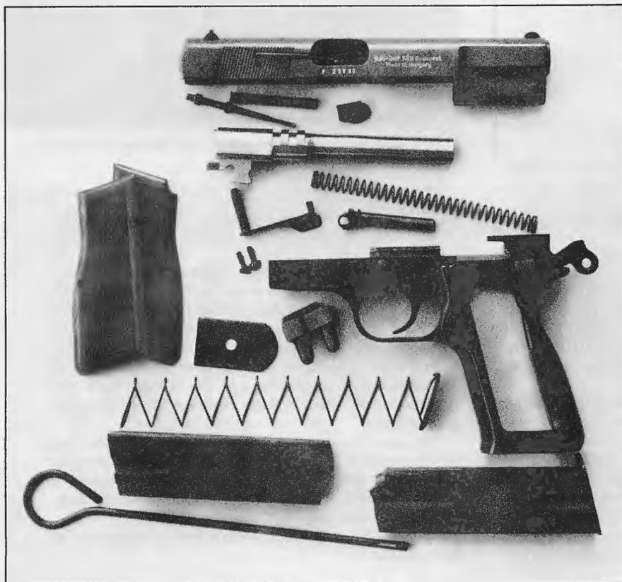
is more evidence of hand-fitting on the PJK-9HP. Its 13-round staggered-column magazine with gray plastic follower remains as difficult to load as the FN original.
