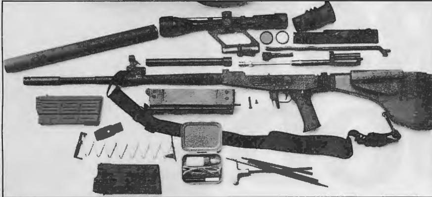
threaded to the barrel. It has three rows of exhaust ports of five holes each positioned to the rear of four transverse compensator cuts arranged two abreast. It can be rotated offset to the right or left to accommodate right- or left-handed shooters (unfortunately, to no avail). It's quite effective but retained by an allen-head set screw which will surely loosen and disappear in the field.
