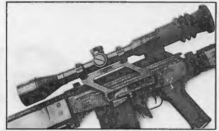
Nimrod 6X40mm scope attached to Galil Sniper Rifle with a quick-release side-rail mount features an excellent Dragunov/RPG-7-type reticle range finder.
