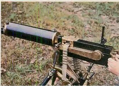
**ABOVE:** Model 1909 Argentine Maxim, caliber 7.65mm, with solid brass water jacket and brass fixtures. **LEFT:** Colt Model 1904 water-cooled Maxim with brass fixtures, originally chambered for the .30-03 cartridge, had been modified to fire .30-06 ball ammo. **RIGHT:** Colt Commercial Browning M38B .30-caliber machine gun with spade grips and wooden ammo box.
