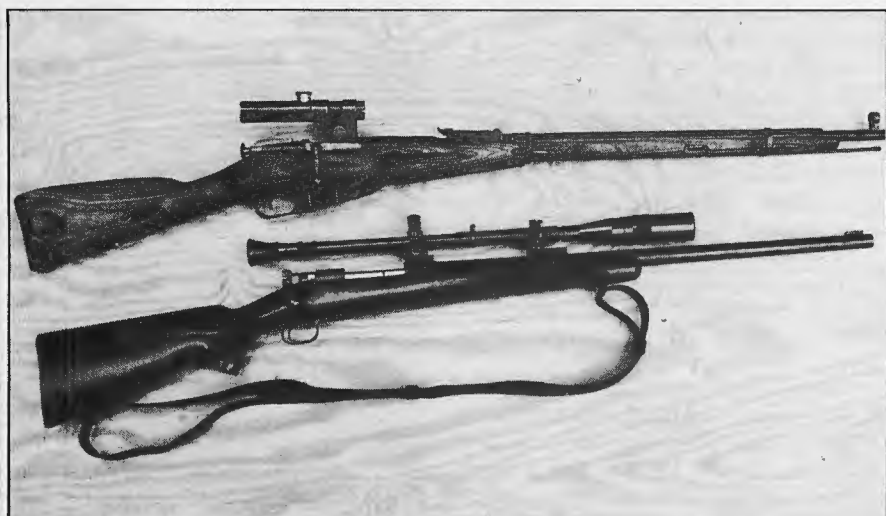
Tools of the trade: Both sides used custom sniping rifles during the Vietnam War. The NVA and VC used the Soviet-made Mosin-Nagant 7.62x55mm rifle with a 3.5X scope (top), while the U.S. Marines used a Winchester Model 70 in caliber .30-06 Springfield with a 10X Unertl scope (bottom). Photo: Hathcock Collection
