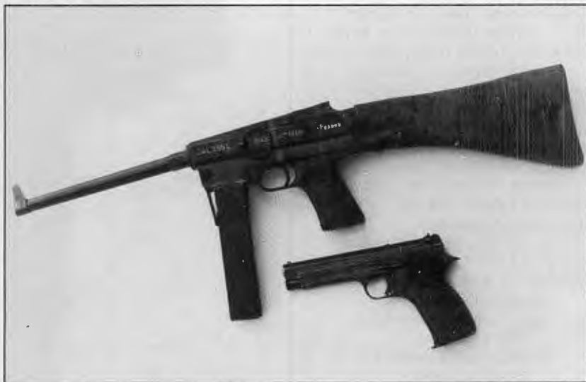
The French MAS Model 1938 SMG and Model 1935A pistol in 7.65mm French Long.
