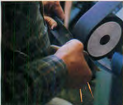
Sparks fly as the belt grinder eats away an unfinished blade.
