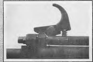
**FA MAS retracting handle and recoil spring cylinder.**
