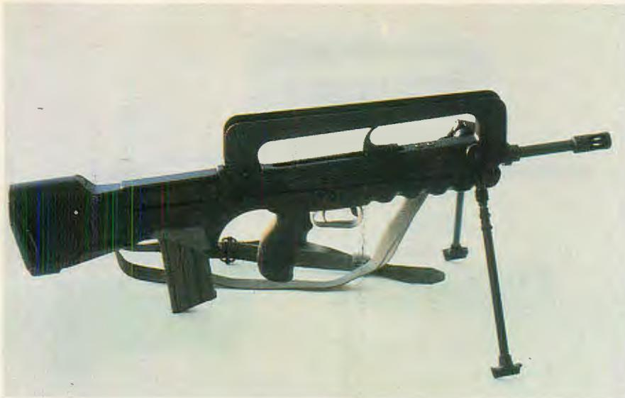
to the barrel and receiver, extends back to the magazine well and cannot be removed. To accommodate the bullpup configuration, the trigger mechanism and pistol grip have been mounted to the lower handguard, forward of the magazine well. The ergonomically-designed pistol grip has three finger grooves and a storage trap which contains a plastic bottle of lubricant.
