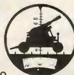
Built-in compass and mil. scale show direction and distance of your target.
