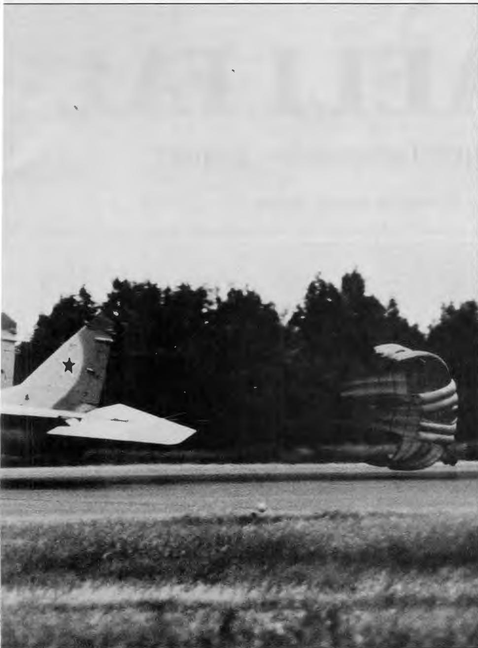
**ABOVE: MiG-29 Fulcrum landing at Finland's Kuopio-Rissala air base. Brake-chute saves wear and tear on brakes and landing gear.**
