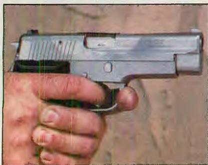
**P220's main changes for blank adaptation are in the barrel, which has to be modified to remove its lock up. Note the difference in the standard barrel, below.**
