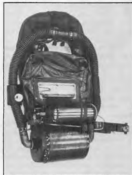
ABOVE: Front view of the oxygen bottle and scrubber. Photo: Bill Stojack
