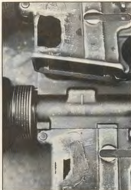
ABOVE: M16A1 rifles worn by salt corrosion from sweaty hands.
