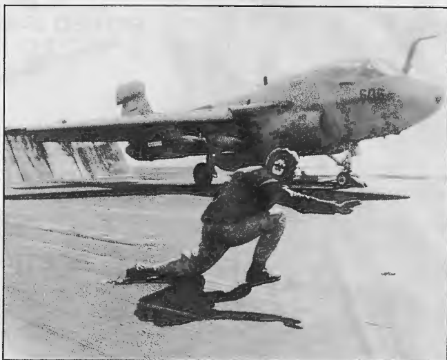
Catapult officer gives the final signal to this EA-6B Prowler to launch from the deck of the USS Saratoga . Photo: Dept. of Defense
