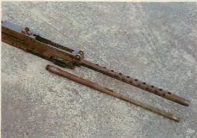
**ABOVE & BELOW:** M3 .50-cal. Browning aircraft machine gun fired until overheated. When barrel slumped an armor piercing projectile sliced through the barrel and jacket.
