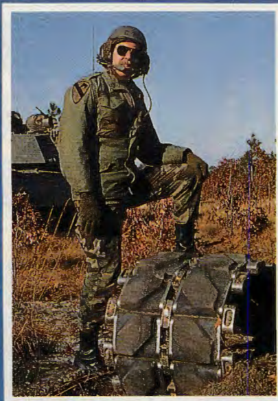
ABOVE: It happens to the best. 2nd Lt. Holland and Platoon Sgt. Ridzelski inspect a thrown track.
