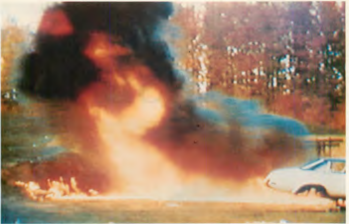
ABOVE: Deliberate attempts were made to ignite an auto gas tank with rifle fire. It worked.
