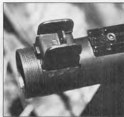
Fixed rear sight with retaining catch to the rear of the sight base. Body is threaded to accept stock.
