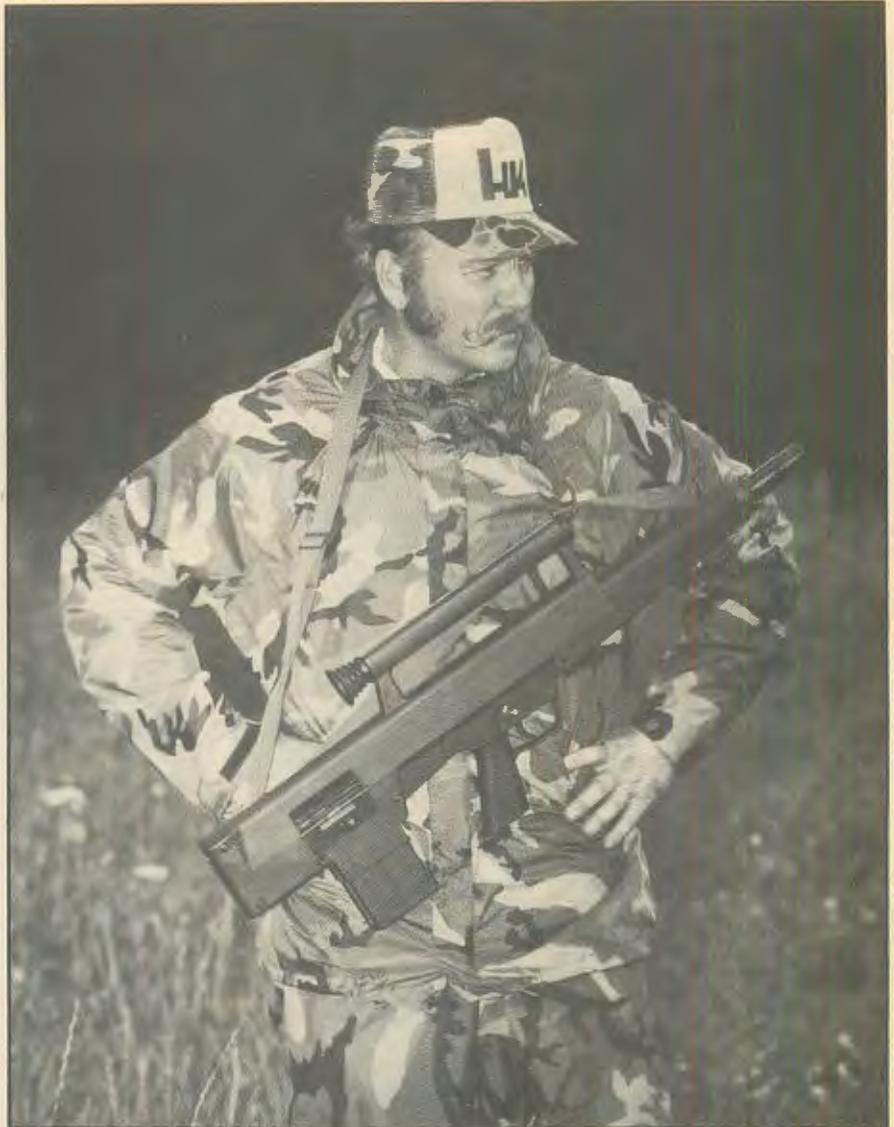
**ABOVE LEFT:** The CAWS can expect to see use as a close-in tactical combat piece for myriad special purpose SWAT uses and military commando operations. **ABOVE:** HK's Close Assault Weapons System will eat new ammo developed by Olin. Star Wars bullpup configuration resembles the HK G11 caseless gun, and is also reminiscent of Steyr's AUG infantry rifle system.
