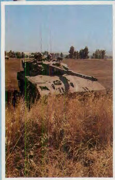
Due to its sleek, sharply angled design, the Merkava can hide effectively behind the proverbial ant hill.
