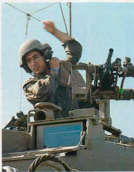
Merkava commander dons flak vest prior to beginning exercise; note the pintel-mounted FN MAG 7.62mm machine gun adjacent to the commander's hatch.
