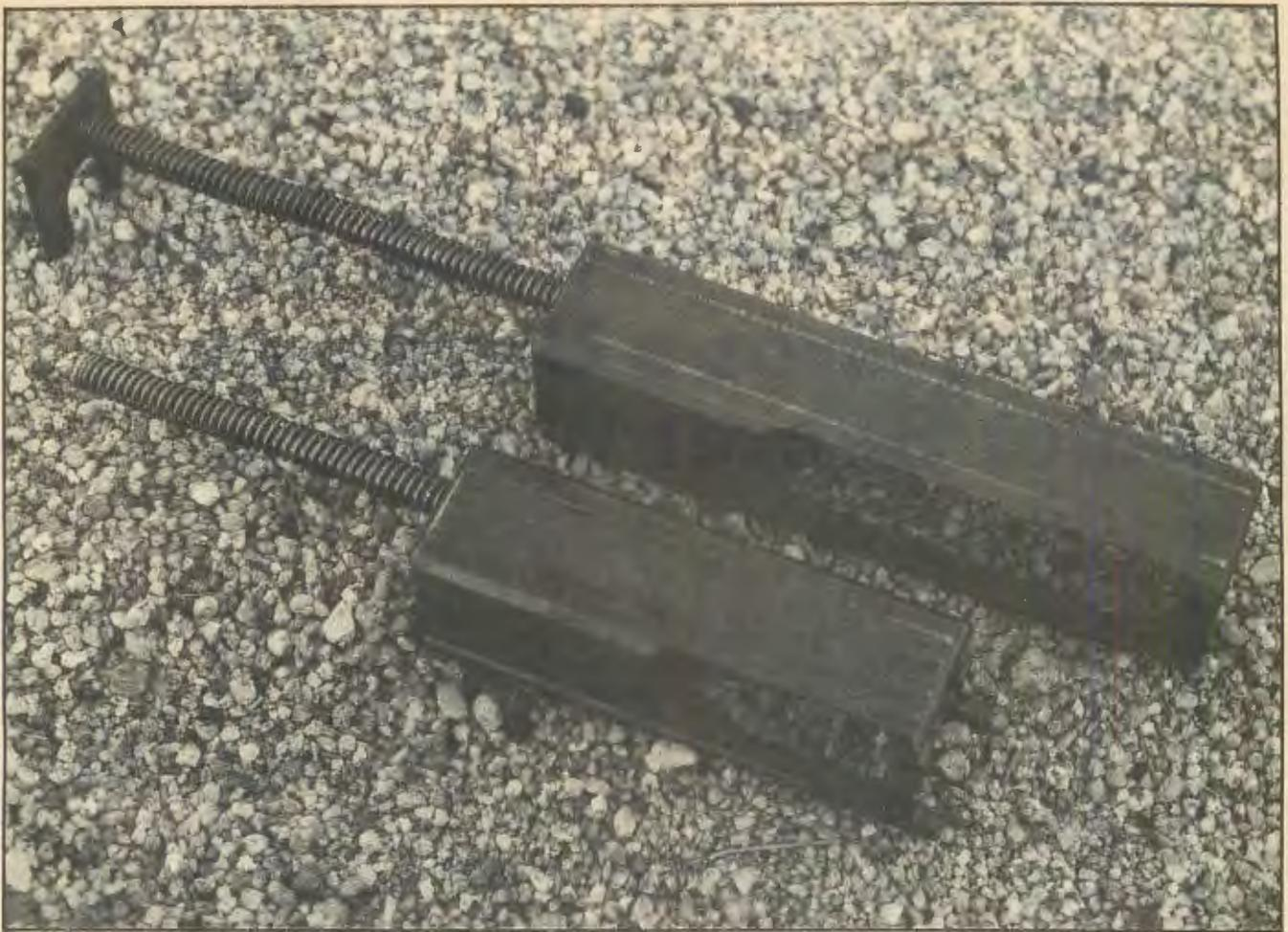
Comparative bolt size of the UZI (top) and Mini UZI. Width, height, extractor and firing pin remain the same on the new square-cut bolt.
