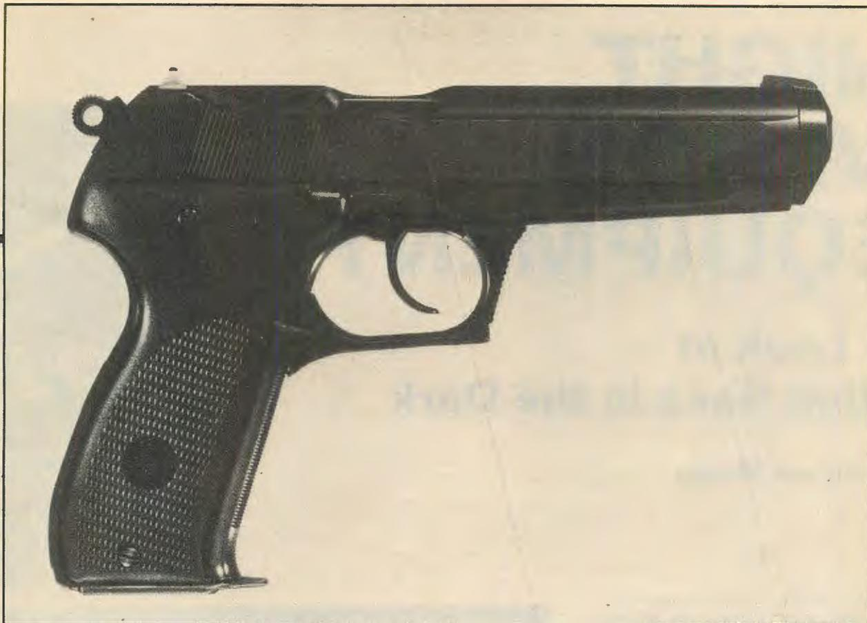
Carbon steel is used throughout the unconventional-looking GB. Only grip panels, trigger guard and magazine spring guide are plastic. Front of trigger guard is checkered for those few who will make use of this feature.
