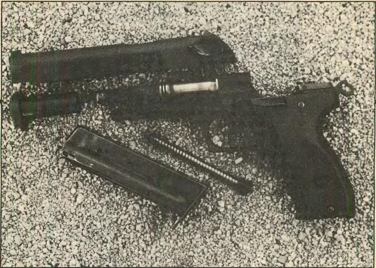
Steyr GB field-strips without tools. No further disassembly is needed, nor should be attempted.
