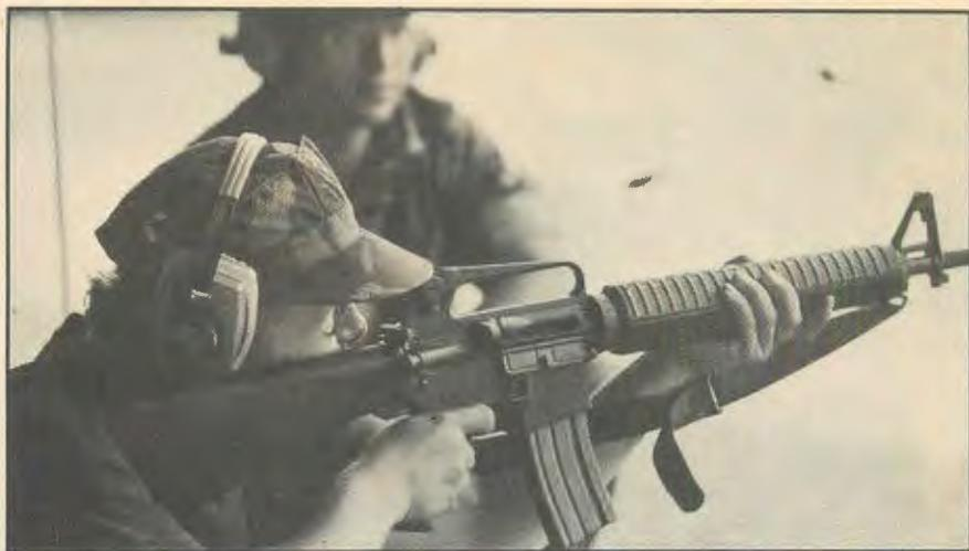
The maximum effective range of the A2 in burst fire is little different than the A1. At 25 meters the rifle averaged a 31x17 inch bullet dispersion.
