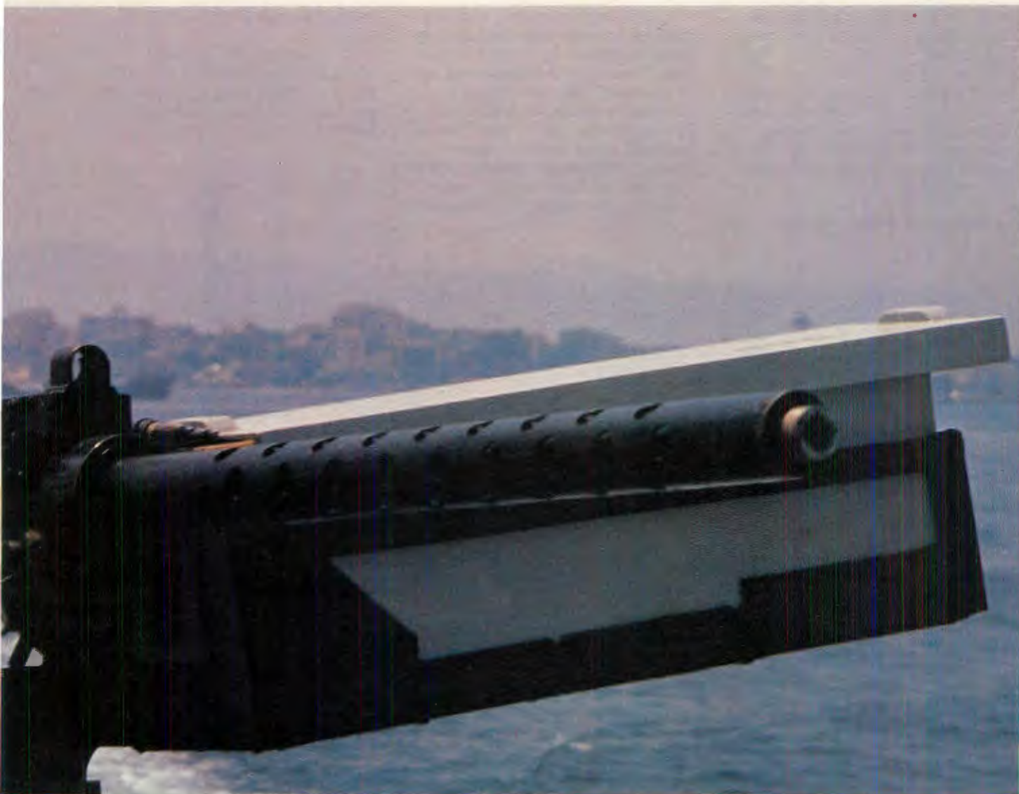
ABOVE: High rate-of-fire Browning .50s provide short-range offense and defense for light-armored patrol boats.
