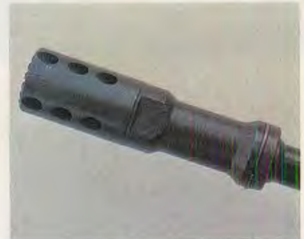
ABOVE: FNC muzzle device patterned after that of the FN FAL accepts the FAL hollow-handle bayonet.
