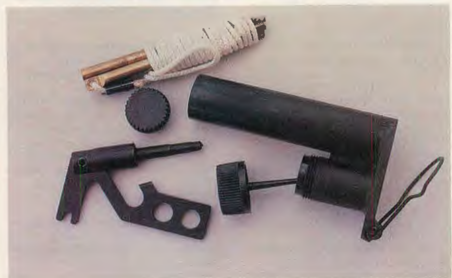
BELOW: FAL Pistol grip cleaning kit and special FNC combo tool for cleaning the gas system.
