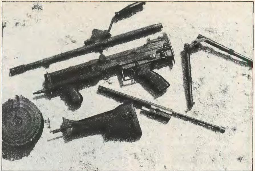
Ultimax 100 SAW — disassembled.
