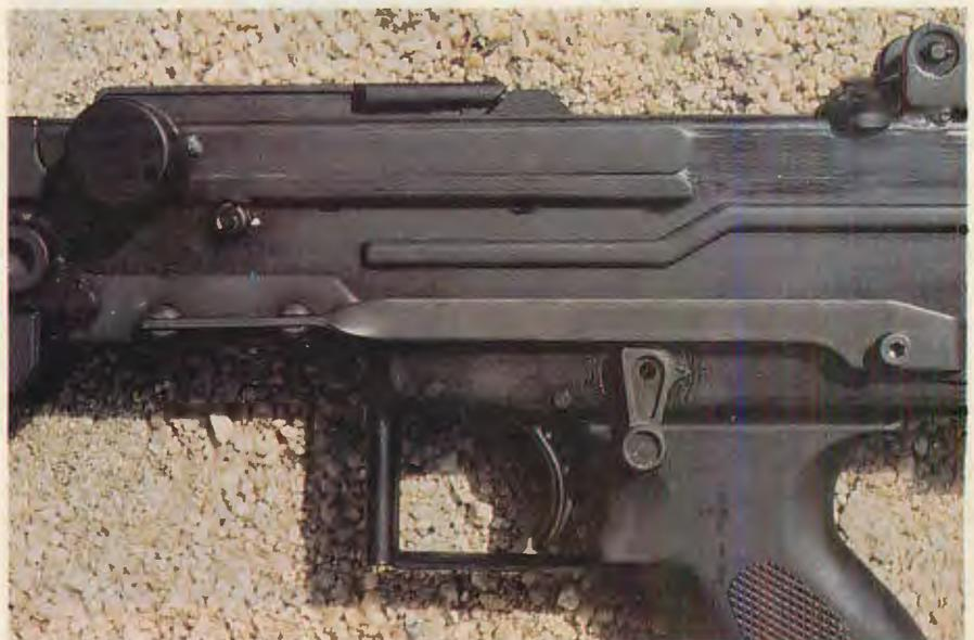
Ultimax 100: left side view. Note that cocking handle knob must be rotated forward before it can be retracted. The magazine latch spring has been mounted outside the receiver.
