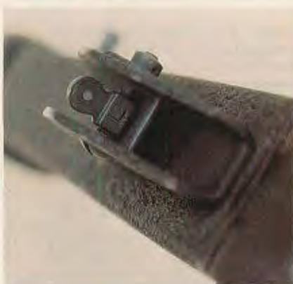
The SAR 80 flip-type, peep-aperture rear sight, taken directly from the M16.
