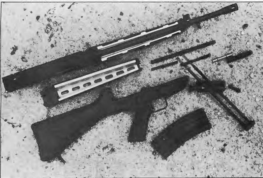
SAR 80 rifle disassembled.
