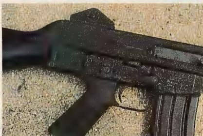
Right side of SAR 80. Note the generous-sized magazine catch release button and peculiar sliding dust cover that does not protect the ejection port.
