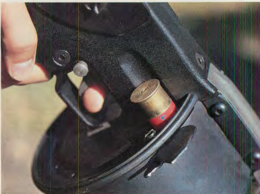
BELOW: The Striker was designed to allow easy loading of shotgun shells into the cylinder.
