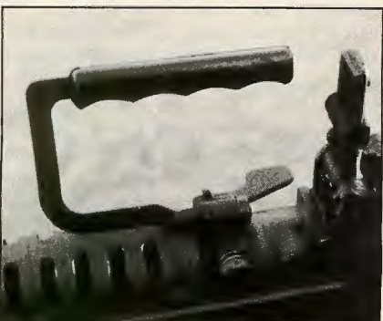
ABOVE: The sights on the M60 are graduated from a distance of 300 meters out to 1,100 meters. LEFT: The carrying handle on the M60 is mounted on the trunnion instead of the barrel where it could make barrel changes easier.
