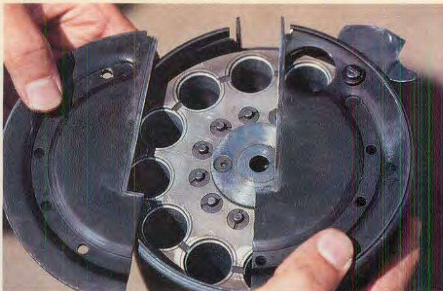
ABOVE: Twelve-shot magazine can be removed by simply disassembling a two-piece plate at the rear of the cylinder.
