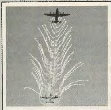
An MC-130 drops flares from fuselage pods over a target. Another gunship follows. Photo: U.S. Air Force
