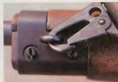
ABOVE: SL7 front barrel band with retaining pins and front sling swivel.
