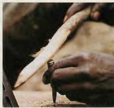
Bullet is carefully pounded back into reloaded case. Round, soft stick prevents igniting primer.
