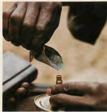
Leaf serves as powder funnel. Propellant is measured by eyeballing level against case neck.
