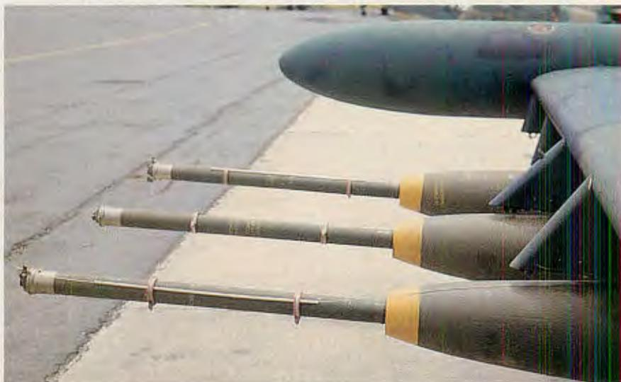
ABOVE: Three-foot fuse extenders on 500-pound bombs ensure detonation above ground level for maximum shrapnel effect. BELOW: Twin M60s in each door of a Huey make it a "gunship." Photos: Dana Drenkowski
