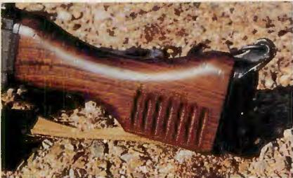
FN MAG 58's distinctive wooden buttstock houses the "hard" buffer with 11 Bellville washers required for a high cyclic-rate machine gun.
