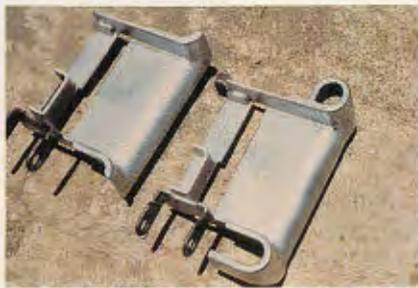
New (left) and old (right) chrome plated feed trays, each with cartridge stops for the DM6 nondistintegrating belt. Both will be soon replaced by a stainless steel investment casting.
