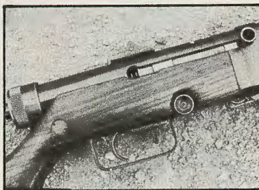
M49/57 closeup shows PPSH-41-type selector inside trigger guard, cross-bolt safety in front of trigger guard, and tubular receiver body. Photo: Peter G. Kokalis
