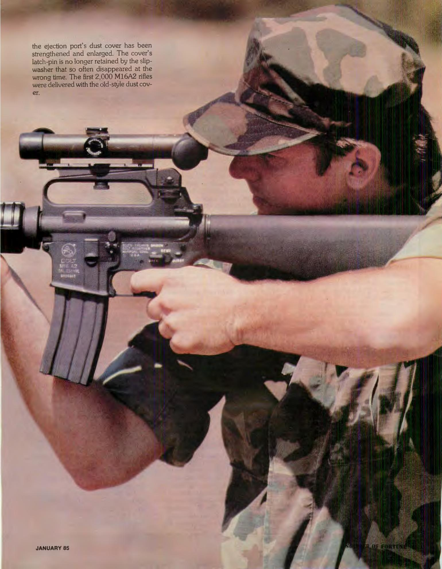
The forward bolt assist has been changed from a casting to a screw machine component with a button-like shape and concentric rings. I have never once personally used or observed anyone using the forward bolt assist in a battlefield. When I inquired of Colt officials why this feature was retained, I was informed that no one requested its removal. And so mutations often pass into the orderly cycle of evolution.
