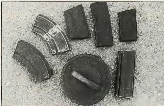
Bren magazines: Left to right, top, .303 magazine, .303 blank magazine, 20-round 7.92mm magazine, L4 7.62mm NATO magazine, 20-round SLR magazine. Below: 100-round drum magazine and Australian 30-round HB FAL magazine.
