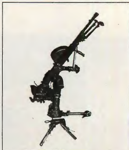
Bren Mk I with 100-round drum and unusual AA mount with geared elevation device. This is not the Mottley mount.
