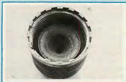
Inside view of silencer's rear nut shows elastomer wipe which limits gas escape, but ruins accuracy.
