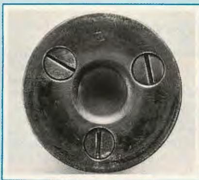
**Heads of tie rods which hold baffles.**
