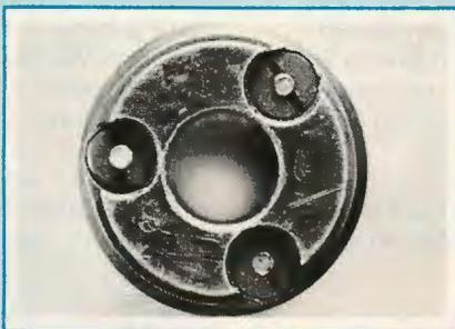
**Slotted round nuts lock baffle assembly to rods.**
