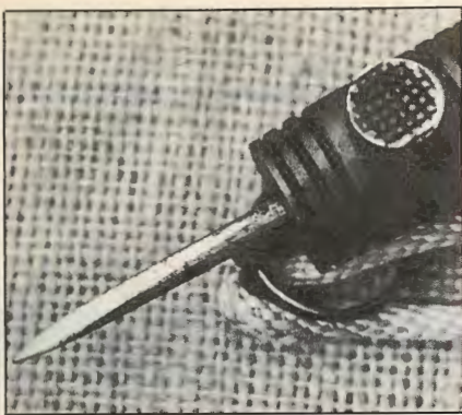
MPCCW close-up shows spike blade and the catch which releases it. Rotating catch also locks blade in place.
