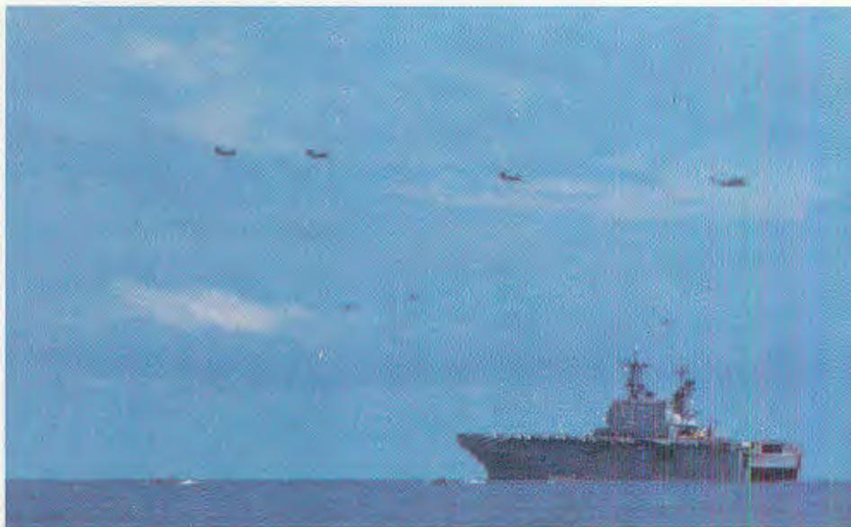
**ABOVE:** Marine CH-46 Sea Knight and CH-53 Sea Stallion helicopters orbit above the USS Nassau off Honduran coast during Big Pine II exercises. Landing Helicopter Assault ships like the Nassau can carry 1,903 troops, up to 19 CH-53 or 30 CH-46s or a mix of these two, and AV-8A Harrier VSTOL jets. They also have a flooding-type loading dock. LHAs, which are actually larger than WWII Essex-class carriers, have a range of 10,000 miles. Photo: Jim Graves
