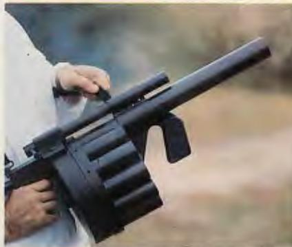
**LEFT:** Developed decades ago as riot-control weapon, 40mm grenade launcher is reborn as MM-1, firing 12 of any mix from smoke, gas, beehive or HE ammo selection. Inserts for 12-ga. are available for 16-lb. revolver.
