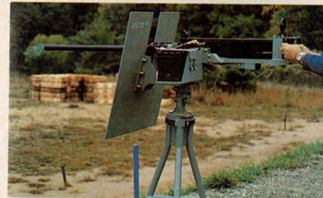
LEFT: Fired from naval deck mount, Browning .50 demonstrates experimental Saboted Light Armor Penetrator (SLAP). LOWER LEFT: GE GAU2B/A double minigun — 12 barrels in all — fires 4,000 rpm of 7.62mm NATO. Fed from 3,000 M21/MAMEE feed/storage system, remote-controlled guns automatically shut off when cone of fire might endanger weapon from excessive traverse.
