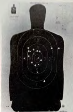
Impact results from six rounds of .38 MMI rapid-fired into a B-34 (reduced scale B-27) silhouette target at a distance of 15 yards.
