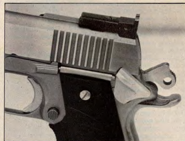
ABOVE: Clean and simple, stripped Score Master shows fewer parts, more stainless than ordinary .45.
