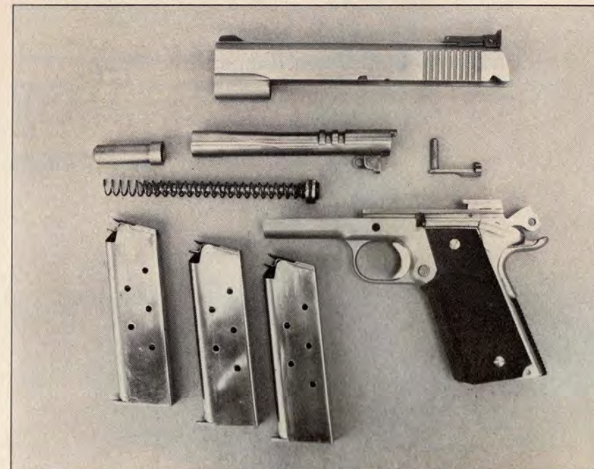
ABOVE: Clean and simple, stripped Score Master shows fewer parts, more stainless than ordinary .45.
