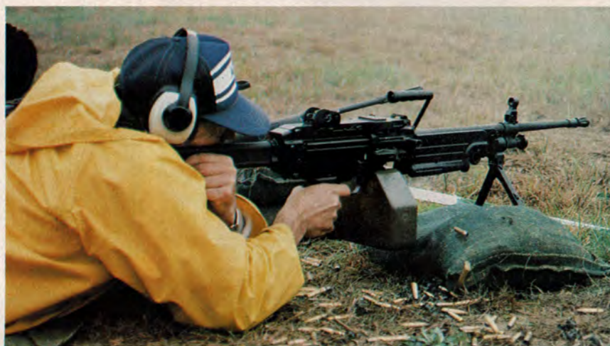
LEFT: Toxic fume levels less than five percent of self-powered MGs make EX-34 Hughes Chain Gun a top competitor in turret or cupola installations.
