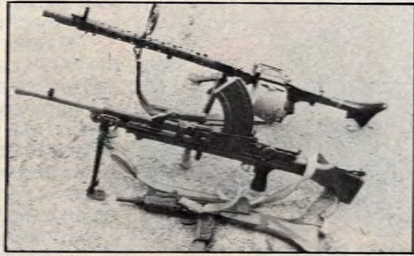
Representing the major types of auto-arms operation (from bottom to top): blowback-operated UZI SMG (Dutch-contract wood stock hand-checked by Israel Galili), gas-operated Mkl Bren gun and recoil-operated (gas-assisted) MG34 (author's collection). Photo: Peter G. Kokalis
