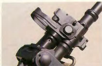
70/78 gas block with lever raised for grenade firing.
