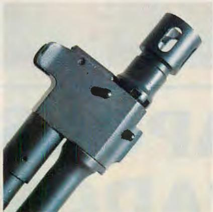
Military 70-series retracting handles are canted upward to allow ambidextrous cocking.
