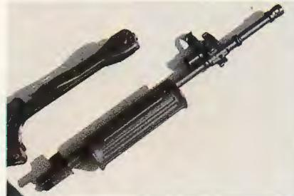
**LOWER LEFT:** Like other 70-series weapons, 70/78's barrel changes in seconds. Disassembly shows forearm and gas block.
