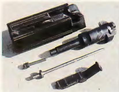
**LEFT:** Beretta 70 bolt assembly, top to bottom: bolt carrier, bolt, firing pin retaining pin, firing pin and retracting handle.
