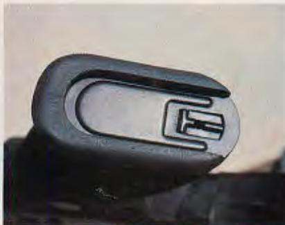
Pistol-grip compartment holds cleaning gear.
